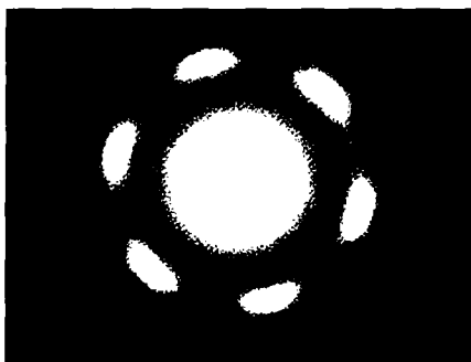
Fig. 3. Electron diffraction pattern from an eight-layer 3(10)OBC film. The plate was purposely overexposed (several minutes instead of several seconds) to reveal the 12 weak, but discernible, herringbone diffraction spots.
